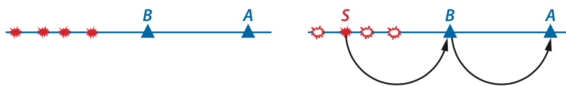
FIGURE 2.1 – Schematic illustration of the sensitivity kernel for the cross-correlation function (from Snieder and Larose (2013)). Left : for surface waves, all sources along the receiver station line contribute to the final cross-correlation function ; right : for body waves, only sources located in a specific area contribute to the final cross-correlation function.
